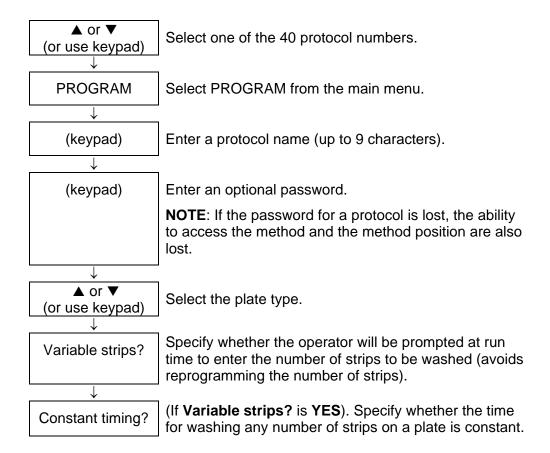
Figure 8. Specifying the Wash Protocol Header
